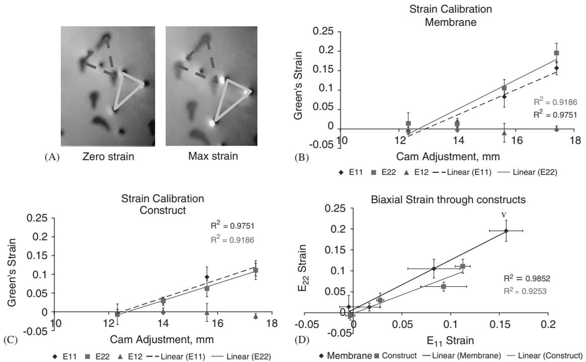
Fig. 3. Strain measurement results: (A) schematic of strain measurement; (B) equibiaxial strain profile at the level of the membrane; (C) equibiaxial strain profile at the free surface of the constructs; and (D) near homogeneous transmission of strain through the thickness of the construct to a maximum of 10%, above which tissue failure ensues. \* $P < 0.05$ .
