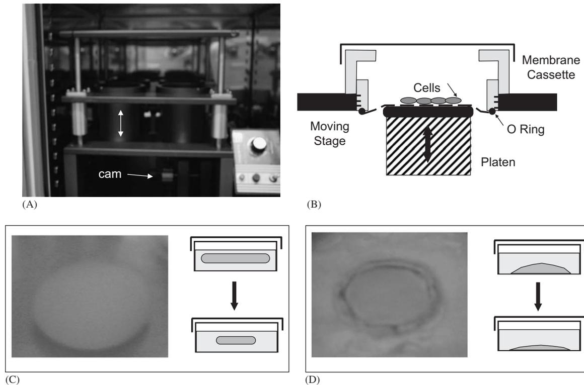
Fig. 1. Experimental systems: (A) the equibiaxial strain device; (B) schematic of the device operation; (C) diagram of the disk model; and (D) diagram of the hemisphere model.
